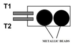
As shown in figure inside SW-520D tilt sensor all we have is two metallic beads. And the output terminals are projected to the inside. When the tilt switch lies horizontally on the plane, the two metallic balls rest on the floor as shown in figure. Under this situation there will no contact between terminals T1 and T2. So T1 and T2 will be open.
